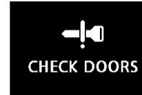
When the ignition switch is in the “LOCK (PUSH OFF)” position, and someone tries to lock the vehicle by pressing the driver’s or front passenger’s door lock/unlock switch while one of the doors is not fully closed, the warning display is displayed and the buzzer sounds for about 3 seconds as a warning, and the doors cannot be locked.
