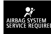
The system checks itself every time the ignition switch is turned to the “ON” position. The SRS warning light will come on for several seconds and then go out.
