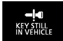
When the ignition switch is in the “LOCK (PUSH OFF)” position, the F.A.S.T.-key is left in the passenger compartment, all the doors are closed, and someone tries to lock the vehicle by pressing the driver’s or front passenger’s door lock/unlock switch, the warning display is displayed and the buzzer sounds for about 3 seconds as a warning, and the doors cannot be locked.
