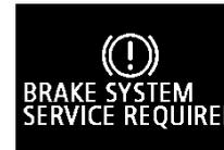
When the ignition switch is turned to the “ON” position, if the brake fluid is low, this warning is displayed.
