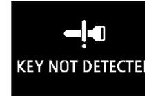
When the ignition switch is in a position other than the “LOCK (PUSH OFF)”, if the door(s) are opened, the F.A.S.T. - key is removed from the passenger compartment, and then the door(s) are closed, the warning display is displayed and the buzzer sounds 4 times as a warning since it’s impossible to verify the ID codes of the F.A.S.T.-key and vehicle.
