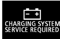
If there is a fault in the charging system, the warning display is displayed on the information screen in the multi-information display. The warning light in the instrument cluster also illuminates.
