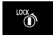
If the driver's door is opened while the ignition switch is in a position other than "LOCK" (PUSH OFF), the ignition switch return reminder buzzer will sound intermittently to remind you to return the ignition switch to the "LOCK" (PUSH OFF) position. The warning display will be displayed on the information screen in the multi-information display.
