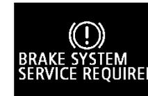
When the ignition switch is turned to the “ON” position, if the brake fluid is low, this warning is displayed.
