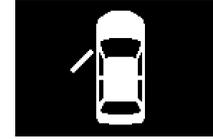
If any of the doors or the rear hatch is not completely closed, this displays the open door or rear hatch.
