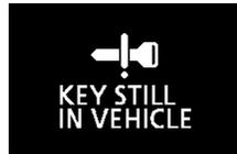
When the ignition switch is in the “LOCK (PUSH OFF)” position, the F.A.S.T.-key is left in the passenger compartment, all the doors and the rear hatch are closed, and someone tries to lock the vehicle by pressing the driver’s or front passenger’s door lock/unlock switch, or the rear hatch LOCK switch, the warning display is displayed and the buzzer sounds for about 3 seconds as a warning, and the doors and the rear hatch cannot be locked.
