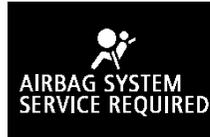
The system checks itself every time the ignition switch is turned to the "ON" position. The SRS warning light will come on for several seconds and then go out. This is normal and means the system is working properly.
