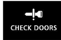
When the ignition switch is in the “LOCK (PUSH OFF)” position, and someone tries to lock the vehicle by pressing the driver’s or front passenger’s door lock/unlock switch, or the rear hatch LOCK switch while one of the doors or the rear hatch is not fully closed, the warning display is displayed and the buzzer sounds for about 3 seconds as a warning, and the doors and the rear hatch cannot be locked.
