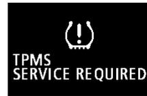
Each tire, including the spare (if provided), should be checked monthly when cold and inflated to the inflation pressure recommended by the vehicle manufacturer on the vehicle placard or tire inflation pressure label. (If your vehicle has tires of a different size than the size indicated on the vehicle placard or tire inflation pressure label, you should determine the proper tire inflation pressure for those tires.)
