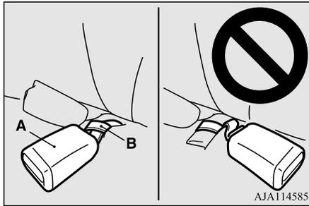
2. Route the seat belt through the child restraint system according to the instructions provided by the child restraint system's manufacturer. Then insert the seat belt latch plate into the buckle. Make sure you hear a "click" when you insert the latch plate into the buckle.
