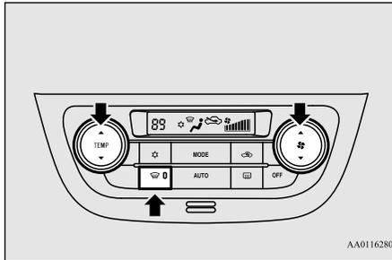
1. Push the defogger switch to change to the “” position.
