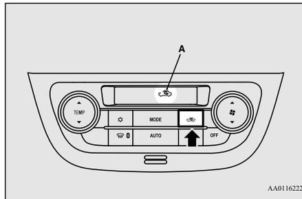
When the air conditioning turns on, the air selection is controlled automatically. When the air conditioning turns off, the air selection automatically goes back to the outside air position.
