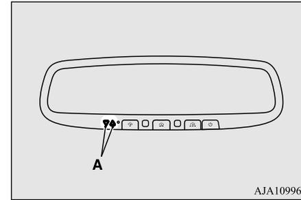
1. Within 5 seconds after successfully programming the garage door opener (refer to “Programming a new HomeLink®” section), both garage door operation indicators (A) will flash rapidly green indicating that the garage door feedback has been enabled. If the indicators do not flash, perform steps 2 and 3 while pressing the HomeLink® button up to the first 10 times after successful programming.
