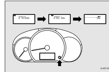
2. Press and hold the multi-information display switch for about 1 second or more to make the wrench symbol start flashing. (If there is no operation for about 10 seconds with flashing, the display will revert to its original indication.)
