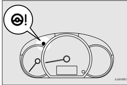
If there is a malfunction in the system, the warning light will come on. Under normal conditions, the warning lamp comes on when the ignition switch is turned to the “ON” position or the operation mode is put in ON, and goes off after the engine has started.
