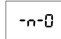
When registration of ID code is complete, the buzzer will sound 3 times and the immobilizer indicator will come on for 30 seconds.
