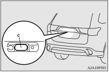
If the open switch is pressed while the power liftgate and all doors are unlocked, the power liftgate will open after the warning buzzer sounds and the hazard warning flasher blinks.
