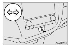
If you press the flasher switch, the front and rear turn signals will flash intermittently, and so will the hazard warning lights. This is an emergency warning system and should not be used when the vehicle is in motion, except for emergencies.
