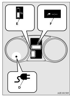
If the charging indicator is not illuminated, charging has not started. Refer to the quick charger user manual.
