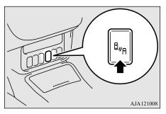
If you turn the BSW ON/OFF, the Rear Cross Traffic Alert (RCTA) also turns ON/OFF at the same time.
