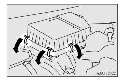
2. Replace the air cleaner filter and put the cover back on in its original position.
