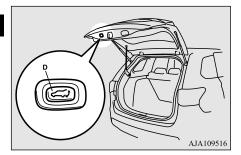
If the close switch on the power liftgate is pressed, the power liftgate will close after the warning buzzer sounds and the hazard warning flasher blinks.
