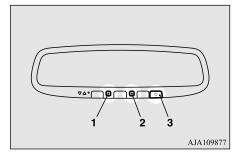
Normally, use the automatic mode. When the operation mode of the power switch is put in ON, the green indicator (1) illuminates and the reflection factor of the mirror is automatically changed.
