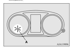
4. The system has entered the armed stage after approximately 20 seconds, when the theft-alarm indicator (A) flashing becomes slower.
