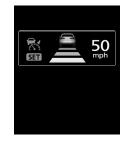
When the front vehicle stops, the ACC will automatically apply the brakes to stop your vehicle.
