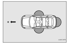
range, even a person not carrying the F.A.S.T.-key can lock and unlock the doors or the liftgate by pressing the driver's or front passenger's door lock/unlock switch, the liftgate LOCK switch or the liftgate OPEN switch.
