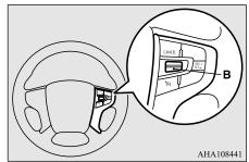
To slow down your speed in small amounts, push down the "SET -" switch (B) for less than approximately 1 second and release it. Each time you push down the "SET -" switch (B), your vehicle will slow down by approximately 1 mph (1.6 km/h).
