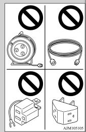
To prevent an electrical shock or fire, do not use a multi type outlet. The grounded line may not work properly and it is not a dedicated type outlet. 4. Press the 8 A/12 A manual selection button (D) on the control box to charge quickly when needed. If selected, the 12 A indicator (E) will illuminate.
