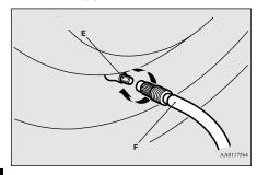
If there is a gap between the tire and wheel, push the tread area toward the center of the wheel to close the gap before running the compressor.
