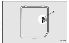
3. Clamp it on the fuse you wish to remove, and pull the fuse straight out from the fuse block.
