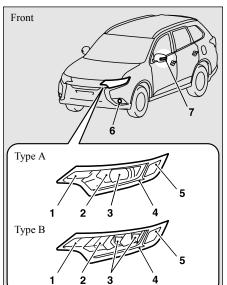
Type A: Halogen headlights type Type B: LED headlights type
