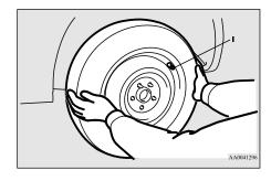
7. Turn the wheel nut clockwise by hand to initially tighten them.
