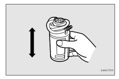
• In cold conditions (when the ambient temperature is 32 °F {0 °C} or lower), thickening of the tire sealant can make the tire sealant hard to squeeze out of the bottle. Warm the bottle between your hands inside
