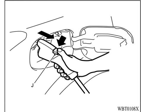
7. When the charging indicator (G) stops blinking, charging is complete. Pull out the normal charge connector while pressing the release button (J).
