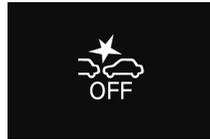
To turn on the FCM again, press and hold the FCM ON/OFF switch. The
