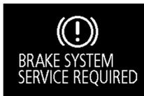
When the ignition switch is turned to the “ON” position or the operation mode is put in ON, if the brake fluid is low, this warning is displayed.
