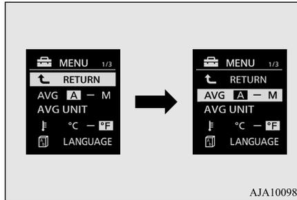
3. Press and hold the multi information display switch (for about 2 seconds or more) to switch in sequence from A or 1 (Auto reset) → M, 2 or P (Manual reset) → A or 1 (Auto reset).
