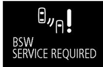
When the warning display appears, the BSW does not operate normally because there are some malfunctions in the system or the sensor. Have the vehicle inspected at an authorized Mitsubishi Motors dealer as soon as possible.
