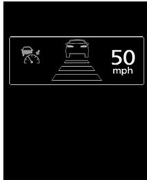
In any of the situations listed below, the ACC control is automatically canceled, a buzzer sounds and a message is shown in the multi-information display.
