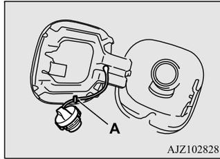
4. Fueling correctly depends mainly on correct handling of the fuel filler nozzle. Do not tilt the nozzle. Insert the nozzle in the fuel tank filler port as far as it goes.
