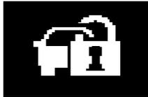
When registration of ID code is complete, the buzzer will sound 3 times and the immobilizer display will come on for 30 seconds.
