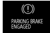
If the Electric parking brake cannot be applied automatically due to the system malfunction, the message will appear on the information screen in the multi information display. Depress the brake pedal.
