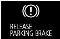
This warning is displayed if the vehicle is being driven with the parking brake still applied. The warning light in the instrument
