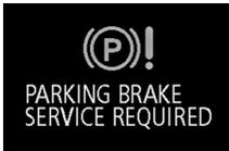
If there is a malfunction in the system, the warning light will come on. In addition, the warning display appears on the information screen in the multi information display.
