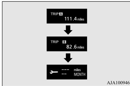
2. Press and hold the multi information display switch (for about 2 seconds or more) to display “” and make it flash. (If there is no operation for about 10 seconds with this indicator flashing, the display returns to the previous screen.)
