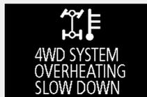
Reduce speed and, if the indicator stops blinking, you may resume normal driving.
