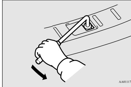
3. Lift up the section of the tire hanger (B) that is marked with the arrow in the illustration and remove it from the hook (C). Then lower it and remove the tire.
