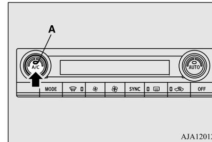
Push the switch again and the air conditioning compressor will stop and the indicator light goes off.
