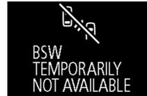
When the warning display appears, the sensor is temporarily not available for some reason such as the environmental condition or increase of the sensor temperature. When the warning display does not disappear after waiting for a while, contact an authorized Mitsubishi Motors dealer.
