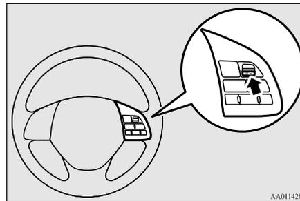
The set indicator comes on, the set speed is indicated and the following distance indicator changes to the ‘active’ display. Also a buzzer will sound.
