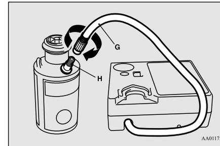
10. Install the bottle onto the compressor.
