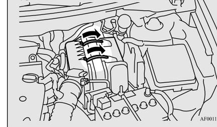
4. Replacing the air cleaner filter and put the cover back on in its original position.
