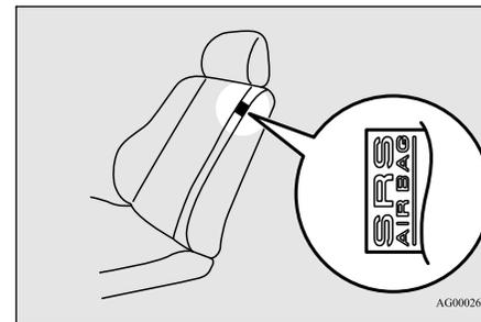
Supplemental Restraint System (SRS) - airbag
