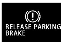
This warning is displayed if the vehicle is being driven with the parking brake still applied. The warning light in the instrument cluster only comes on when the parking brake is applied.
