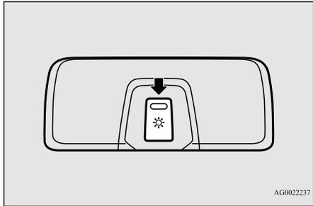
The brightness of the sunshade illumination can be adjusted to 3 different levels when the ignition switch or the operation mode is in ON or ACC.
