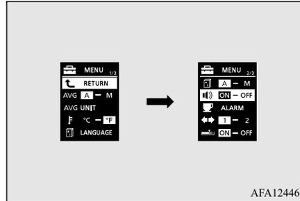
3. Press and hold the multi-information meter switch (for about 2 seconds or more) to switch in sequence from ON (operation sound on) → OFF (operation sound off) → ON (operation sound on).
