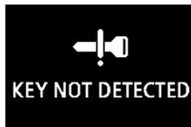
When the operation mode is in any mode other than OFF, if the door(s) are opened, the F.A.S.T.-key is removed from the passenger compartment, and then the door(s) are closed,
