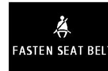
A tone and warning light are used to remind the driver to fasten the seat belt.
