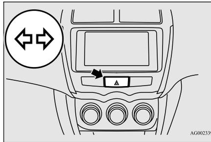
If you press the flasher switch, the front and rear turn signals will flash intermittently, and so will the hazard warning lights. This is an emergency warning system and should not be used when the vehicle is in motion, except for emergencies. If you need to leave your vehicle, the flashers will keep working after the ignition switch is removed or the operation mode is put in OFF.
