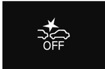
To turn on the FCM again, press the FCM ON/OFF switch. The
