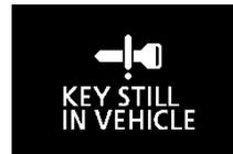
When the operation mode is in OFF, the F.A.S.T.-key is left in the passenger compartment, all the doors and the liftgate are closed,
