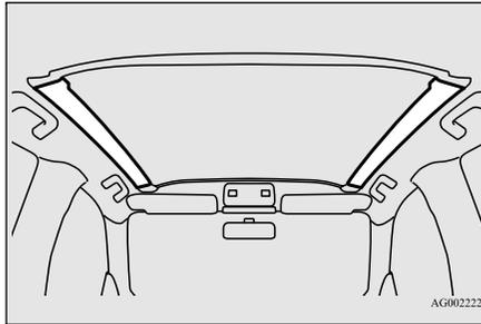
The sunshade illumination turns on when the ignition switch or the operation mode is in ON or ACC.
