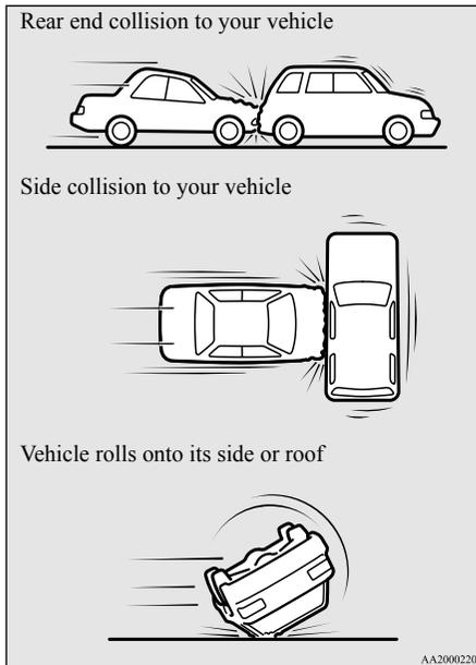
**The front airbags and driver's knee airbag MAY DEPLOY when**
