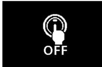
When the operation mode is in any mode other than OFF, and someone tries to lock the vehicle by pressing the driver's or front passenger's door lock/unlock switch, or the liftgate LOCK switch, the warning display is displayed and the buzzer sounds for about 3 seconds as a warning, and the doors and the liftgate cannot be locked.
