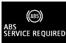
If there is a malfunction in the system, the anti-lock braking system warning light will come on and the warning display will appear
