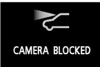
When the sensor performance returns, the FCM functions will resume operation. If the message continues showing, there is a possibility that the sensor has a malfunction. Contact an authorized Mitsubishi Motors dealer for inspection of the sensor.
