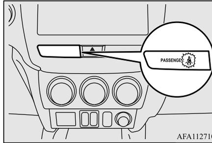
When the ignition switch is turned to the “ON” position or the operation mode is put in ON, this indicator normally comes on and goes off a few seconds later. The light comes on when a person sits on the front passenger seat but does not fasten the seat belt. It goes off when the seat belt is subsequently fastened.
